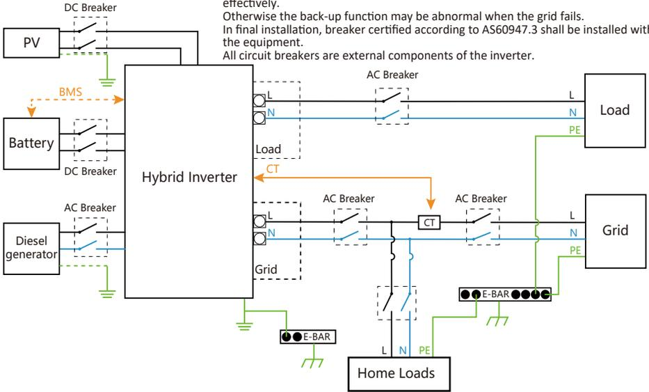
This diagram is an example for application that Neutral connects together with PE in distribution box.
