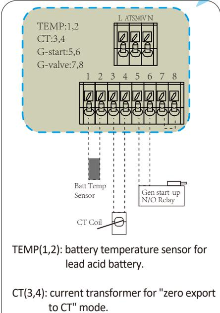
TEMP(1,2): battery temperature sensor for lead acid battery.
