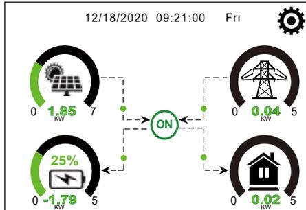
1.The icon in the center of the home screen indicates that the system is Normal operation. If it turns into "comm./FXX" , it means the inverter has communication errors or other errors, the error message will display under this icon(FXX errors, detail error info can be viewed in the System Alarms menu).
