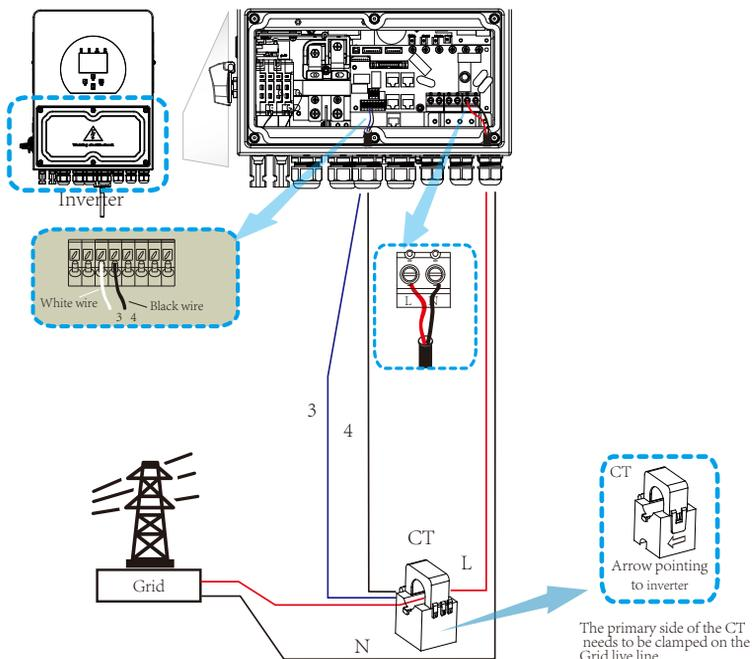
**\*Note:** when the reading of the load power on the LCD is not correct, please reverse the CT arrow.
