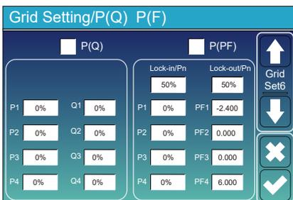
**P(Q)**: It is used to adjust the inverter reactive power according to the set active power.
